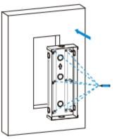
Install the flush-mounted box.
