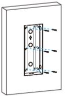
Place the flush mounting bracket inside the box and fasten it using the supplied M4 screw.
