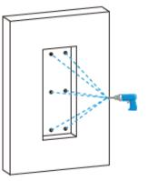
Secure the box by fastening screws through the six mounting holes in the bottom.
