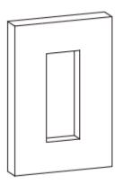
Create a wall opening based on the external dimensions provided on page 1. Note: the listed dimensions represent the actual size of the box. The opening should be slightly larger (by a few millimeters) to allow for proper fitting.
