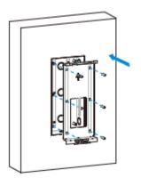
Before installing the door phone, the flush mounting bracket must be mounted inside the box.
